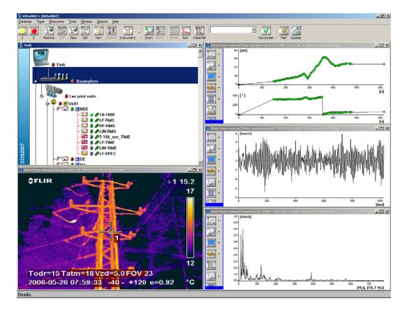
Graphs of spectra, cursor – single, harmonic, side-band, delta, delta max, band-cursor, trend-cursor, x axis – lin, log, OKT/1, OKT/3, Hz, RPM, order, y axis – lin, log, auto or fix scaling, grid, zoom, move – dynamic or manual, automatic or fix scaling, marks – local maximum, select of unit – acceleration, velocity, displacement, derivation and integration of signal, view – amplitude, phase, real/imag, trend, polar trend, waterfall diagram, process values, edit data function
